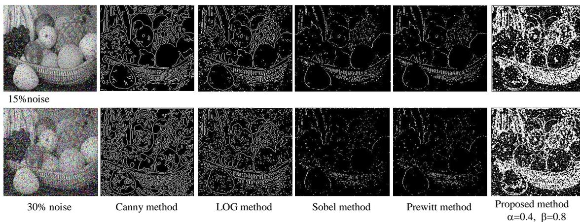
**Figure 6: Performance of Proposed Edge Detector for Fruits image with Various salt and pepper**
