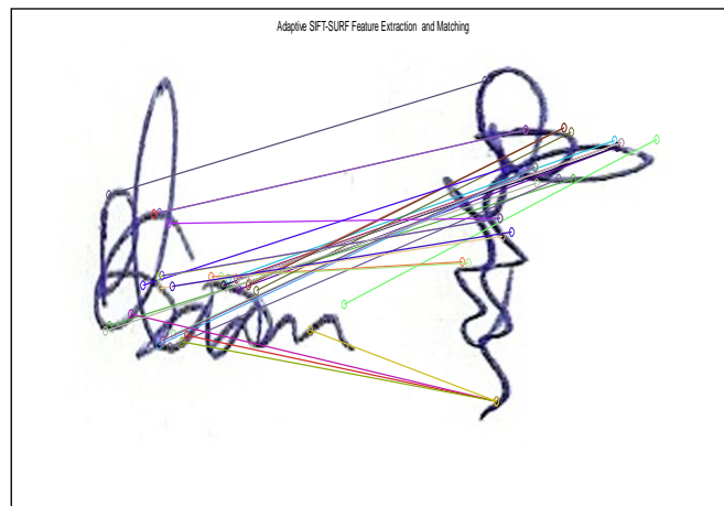
Figure 5 Sample of the same signature as in figure 4 using Adaptive SIFT-SURF algorithm
