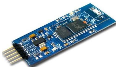
Figure 2. The Bluetooth module (BlueLink)
