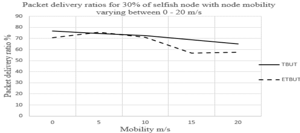
Figure 7: Packet delivery ratio, for 30% selfish node with node mobility varying between 0 - 20 m/s.
