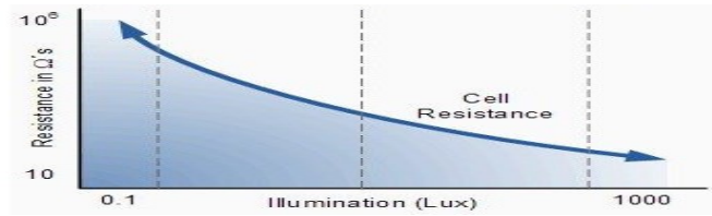
Figure 9. The LDR resistance versus the illumination
